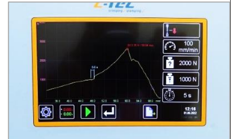
Display of the measurement curve in real time with zoom function
